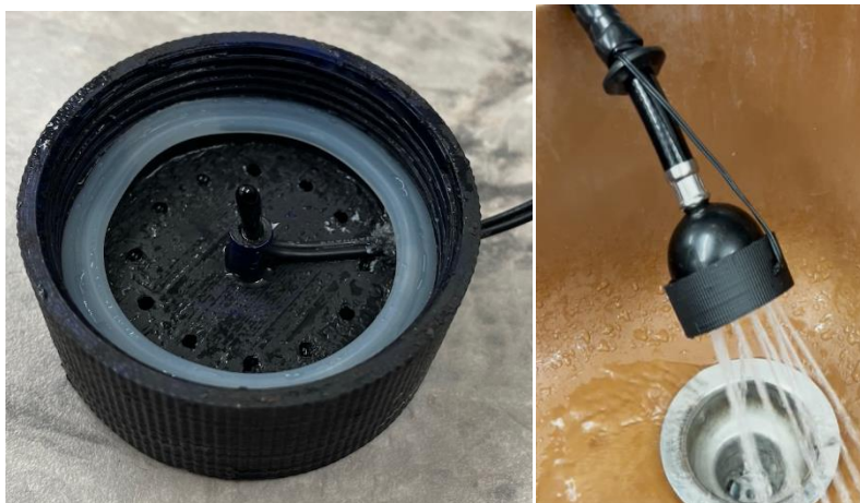
Figure 5.3: Final Showerhead System with Implanted Thermistor
