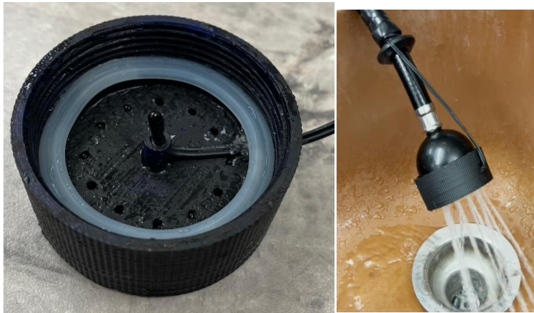
Figure 1.3: Final 3D Printed Showerhead System with Implanted Thermistor
