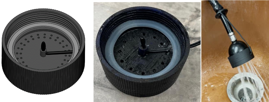
Figure H.22: Final 3D Printed Showerhead System with Implanted Thermistor
