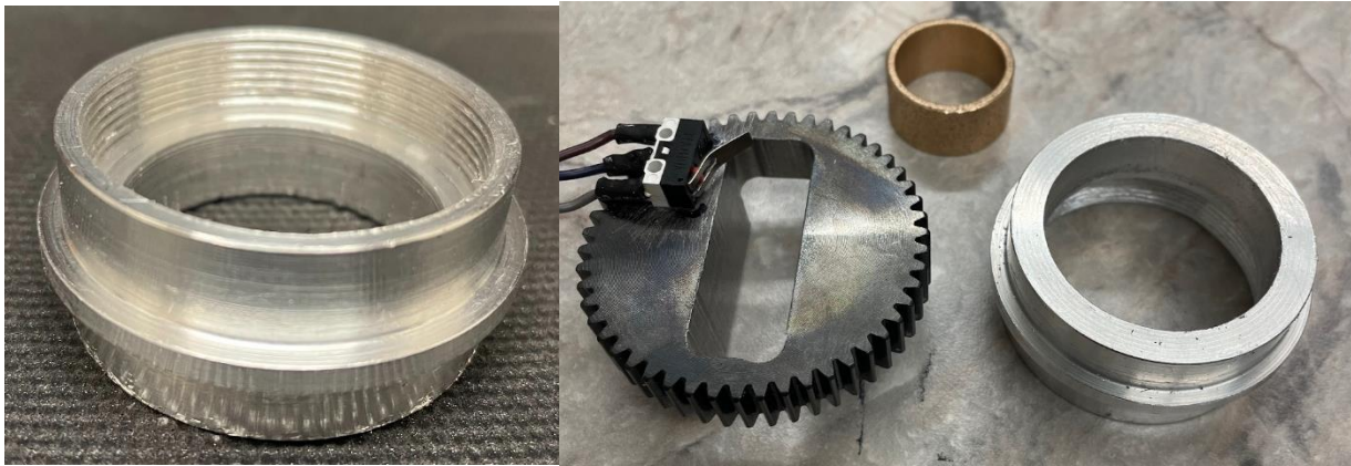
Figure 5.1: Shaft Coupler and Other Machined Parts
