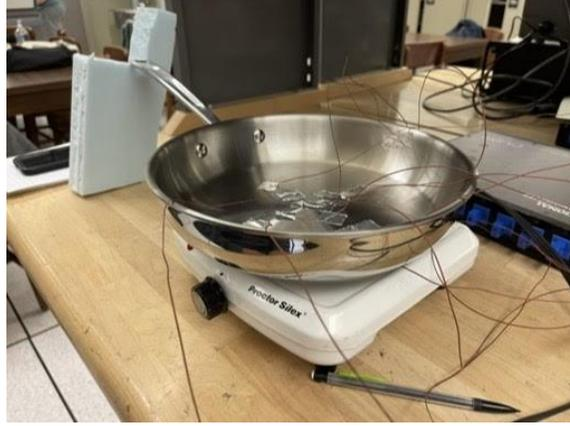
**Figure 3.** The final setup for the pan (stainless steel featured above). In this assembly, thermal tape was used to adhere each thermocouple to the pan.
